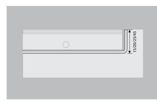
emco dirt collection wells are required to counter the increased dirt levels in heavily frequented entrance areas. When combined with the matching emco entrance mat, they form a closed system which reduces dirt transference and protects adjacent indoor floor coverings.
