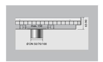
emco dirt collection wells are required to counter the increased dirt levels in heavily frequented entrance areas. Together with the emco MARSCHALL entrance mats combined with a grid and support profile in a narrow arrangement (not when combined with a scraper bar or brush strip), they form a robust unit which is unbeatable in terms of effective cleansing, high load capacity and practicality.
