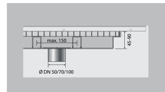
emco dirt collection wells are required to counter the increased dirt levels in heavily frequented entrance areas. Together with the emco MARSCHALL and emco Plaza entrance mats combined with a grid and support profiles in a narrow arrangement (not when combined with scraper bar or brush strip), they form a robust, unbeatable unit in terms of effective cleaning, high load capacity and practicality.
