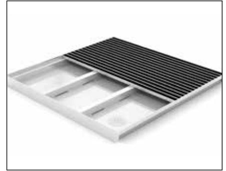
The support for the entrance mat is incorporated into the well. A separate installation frame is therefore no longer necessary. The entrance mat and well form a single unit and are 100% flush with each other, even in special shapes.
